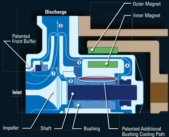
The T-Mag™ Mag-Drive pumps in the 1/2 HP (0.40 kw) through 5 HP (3.75 kw) sizes comes standard with a patented additional fluid flow path around the bushing. This additional path allows the process fluid, or air, to cool the bushing of the impeller from the outside, while continuing to offer the internal spiral cooling
